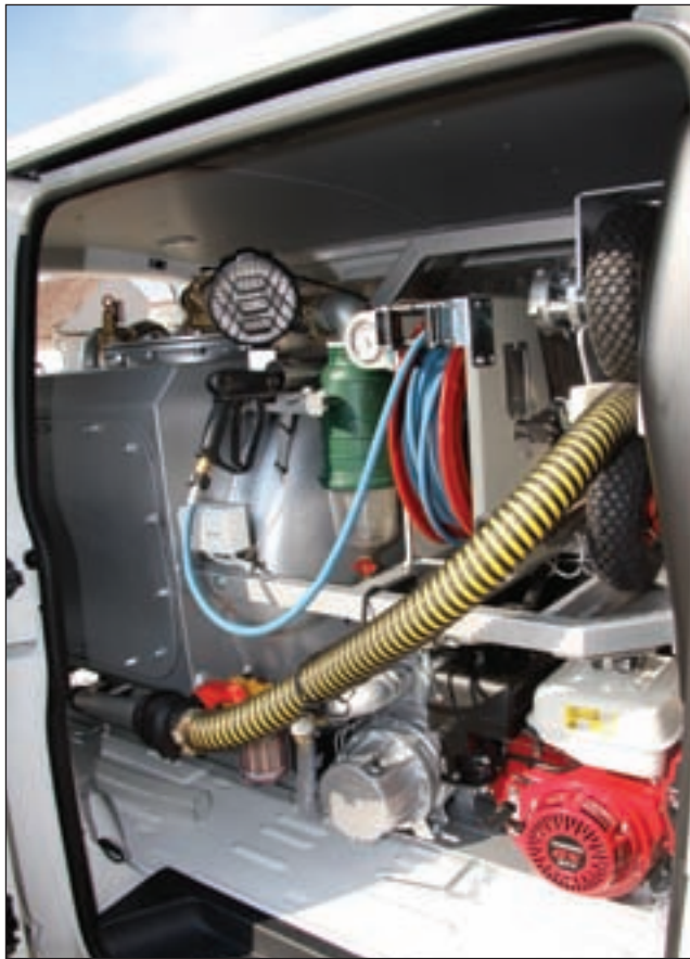
Because of high fuel costs and tight European city streets, Johnny Servis employs small Volkswagen service vans. This one carries a 200-gallon waste, 50-gallon freshwater slide-in unit from Czech company IBOS. The photo at left shows the pump hose and pressure washer. The trucks get 20 mpg.
