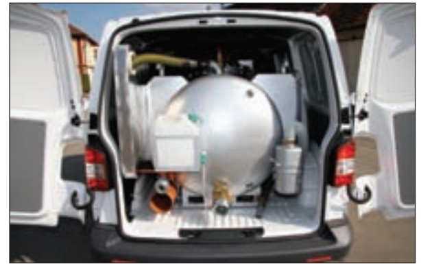
Because of high fuel costs and tight European city streets, Johnny Servis employs small Volkswagen service vans. This one carries a 200-gallon waste, 50-gallon freshwater slide-in unit from Czech company IBOS. The photo at left shows the pump hose and pressure washer. The trucks get 20 mpg.
